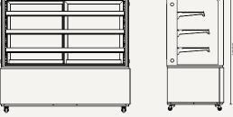
Temperature set range: +2°C to +6°C **Gross/net weight:** 269.5/211 kg
