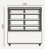
Temperature set range: +2°C to +6°C **Gross/net weight:** 229.5/180 kg Energy consumption in 24h: 8.374 kWh
