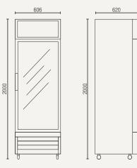
Gross volume: 400 L Exterior dimensions in mm: 606w x 620d x 2000h Number of adjustable shelves: 4 Temperature set range: 0°C to +10°C Gross/net weight: 98/83 kg Energy consumption in 24h: 4 kWh
