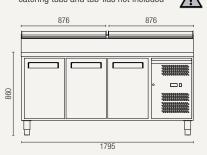
Allow min. 100mm clearance for instalation,
